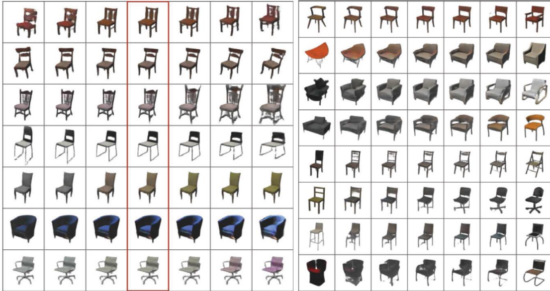
Figure 13. Chair exemplars generated by a network deploying “deconvolution” and “unpooling” operations. On the left are arrayed similar chair exemplars generated by the network by varying nuisance parameters (from top: translation, rotation, size, stretch, saturation, brightness, color), and on the right a range of novel intermediate exemplars between two distinct chair exemplars. (Images reproduced from Dosovitskiy, Springenberg, & Brox, 2015).
