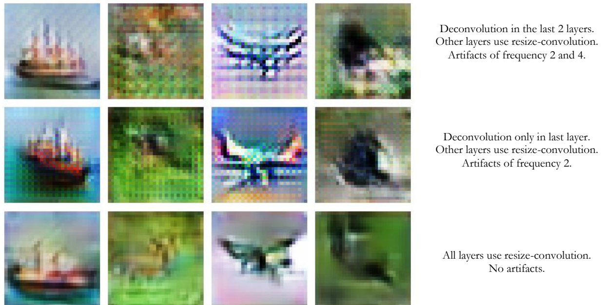
Figure 14. Examples of checkerboard artifacts produced by image deconvolution with and without corrective measures. Specifically, they advocate for an alternative deconvolution method—“resize-convolution”—that reshapes images to fit kernels before attempting to reverse the convolution operation (figure reproduced from Odena et al. 2016).
